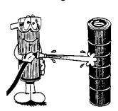
nozzle to wash down the filter element. Work from the top down, holding the nozzle at a 45 degree angle, and wash all the pleats with emphasis between
