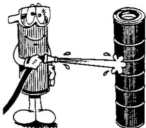
nozzle to wash down the filter element. Work from the top down, holding the nozzle at a 45 degree angle, and wash all the pleats with emphasis between
