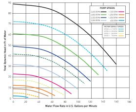
NOTE: The charts above demonstrate performance rates at factory preset speeds of 750 RPM, 1560 RPM, 2350 RPM and 3110 RPM. However, flow rates can also be custom programmed between the ranges of 400 RPM and 3450 RPM.
